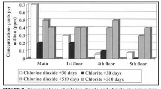
**FIGURE 2.** Concentrations of chlorine dioxide and chlorite at various locations throughout the building after 30 and 510 days of operation of the system. At 30 days, levels were higher at the main than on the first and upper floors; however, this difference had decreased markedly by day 510.
